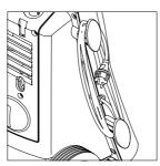
To avoid accidents, the electric cable and the high pressure hose should always be winded carefully up.
